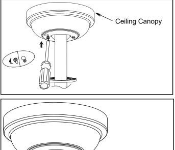
**Step 2:** Securely attach and tighten the ceiling canopy screw cover over the shoulder screw heads in the hanger bracket utilising the key slot twist-lock feature.
