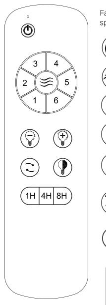
Fan Speed: Press and release immediately to turn on and set fan speeds. Number 6 is the highest speed and Number 1 is the lowest.
