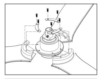
**Step 2:** Place the fan housing over the motor assembly. Align the 6 holes on the fan housing with the holes on the downrod assembly. Securecly attach the fan housing to the motor assembly using the 6 fan housing set screws supplied.
